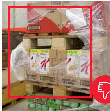
Torn shrink film due to non-compliance with dimensions
