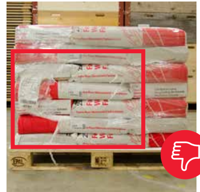
Torn shrink film due to non-compliance with dimensions
